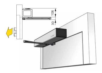
Sliding rods with pushing function Lintel installation
