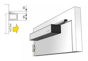
Sliding rods with pulling function Lintel installation
